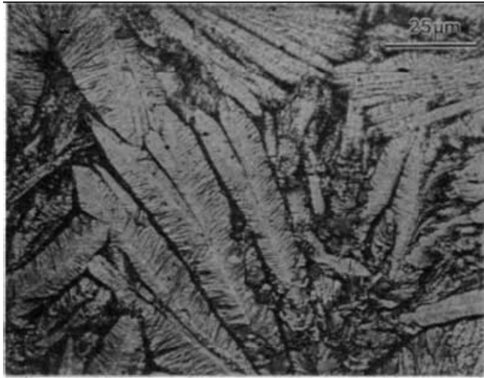
Figure I.6 Reflection optical micrograph of lamellae in isotactic polypropylene arranged in feather-like structures. [8]
