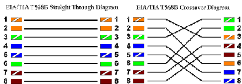
Figure 3 - Wiring of each standard
