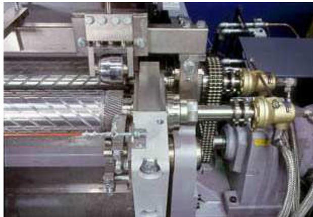
Fig. 3: Granulation unit at the end of a shear roll
