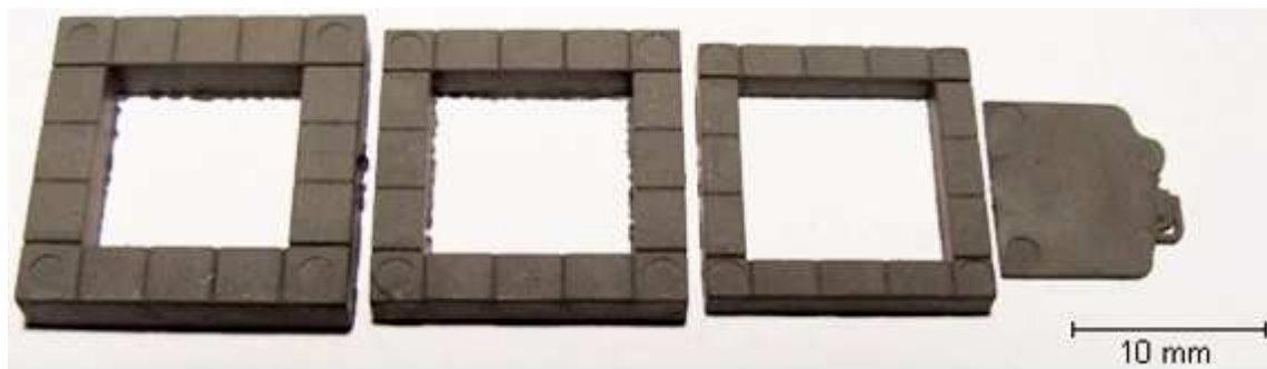
Fig. 34: Testing specimen made of polyMIM ® 316L feedstock
