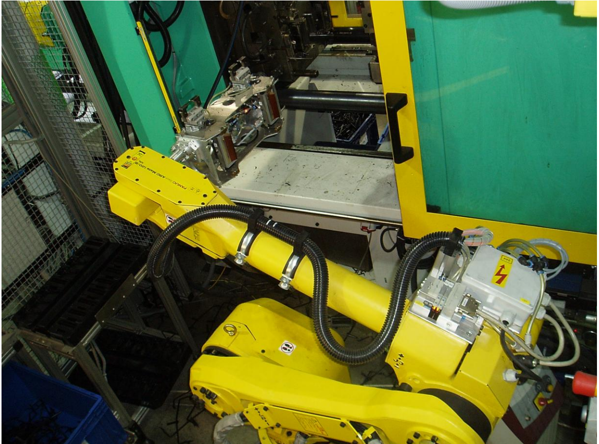
Obr. 23 Robot Fanuc Robot ARC Mate 120 iB 10L [24]
