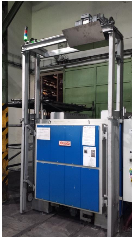
Figure 26 – Furnace for external preheating (own processing)
