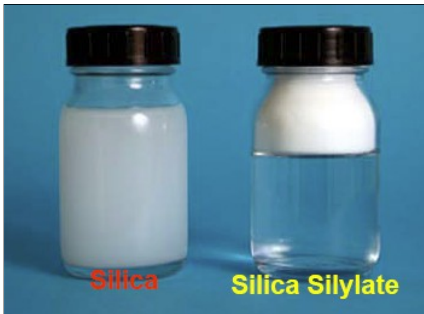
Fig. 11: The difference between hydrophilic silica and hydrophobic silica silylate (the amount of water and dust is always the same). (Borrowed from [20])
