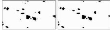
Fig. 1: An illustration of a noise removing from prints – the small dots and speckles in the left part are erased.
