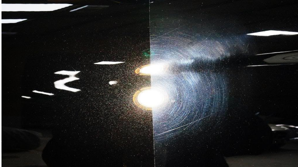
Figure 6 Paintwork after / before polishing (www.exclusivecarcare.co.uk)
