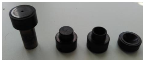
Figure 20: Photo of used capillaries, namely with L/D ratio: 40/2; 20/1; 10/0.5 and orifice 0.1/1 mm
