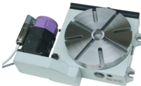
Obr. 38 Otočný stůl IS 160 [22]
