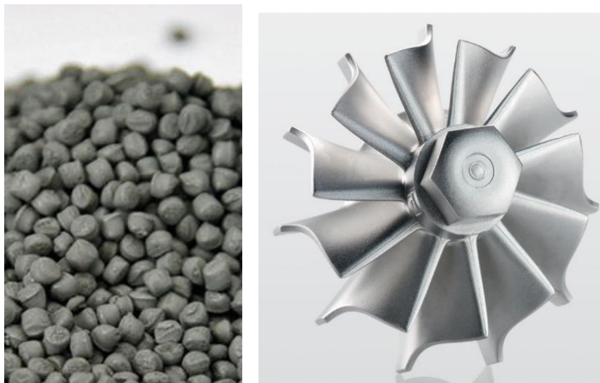
Figure 2. Pelletized PIM feedstock (left) and turbocharger rotor made using PIM technology (right) [13].
