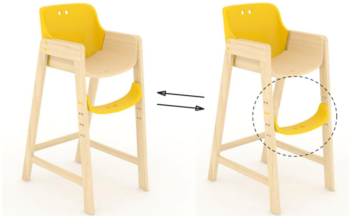
Figure 53. The adjustable footrest of the high chair.
