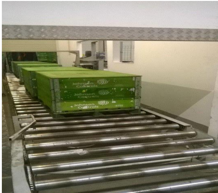
Figure 27: Starting point of strapping machine
