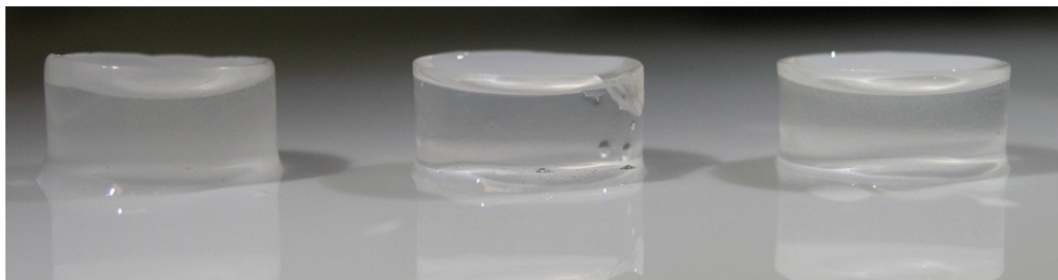
Figure 1: Image of the hydrogel in the swollen state [8].
