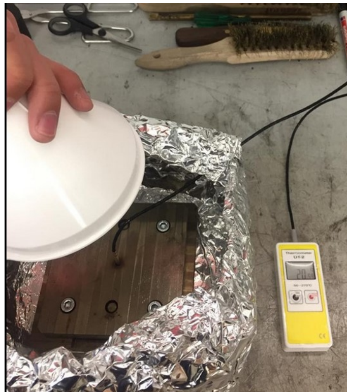
Figure 49 Cooling of the testing mold and testing sample
