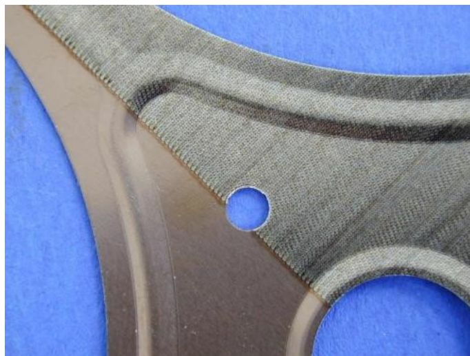
Figure 15 Laser surface preparation (25)
