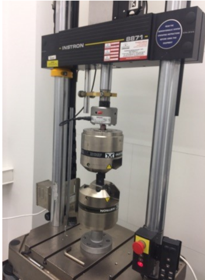
Figure 38 Testing device Instron 8871 (27)
