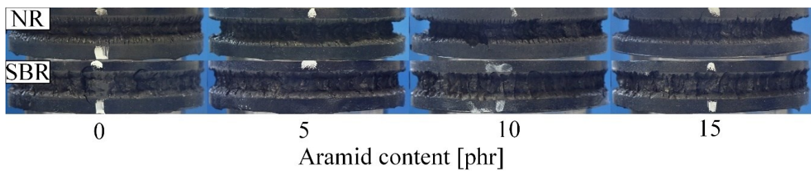
Figure 34: Images of worn NR and SBR samples for different aramid content.
