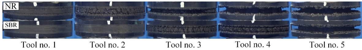
Figure 30: Images of worn NR and SBR samples for different impacting tools.
