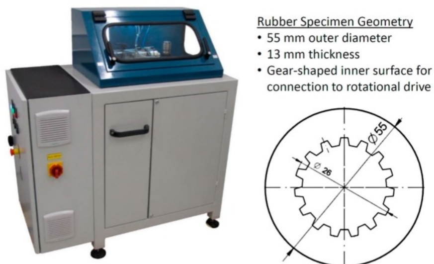
Figure 15: Photograph of instrumented chip and cut analyser (left) and diagram of rubber sample geometry (right). [11]
