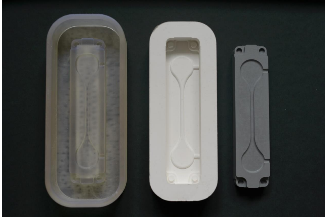
Fig. 40 - 3D printed model (left), negative silicon mold (middle), final insert from epoxy resin (right)
