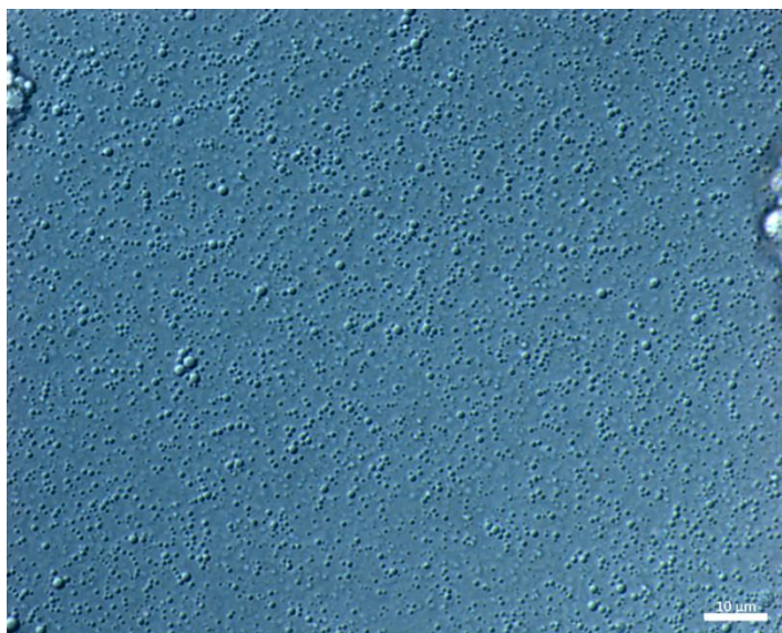
Fig. 7.5 Optical microscopy (magnification 20×) of BC emulsions with o/w 20/80 prepared with 1 wt% CAS while using sonication. Scale bar is 10 μm.
