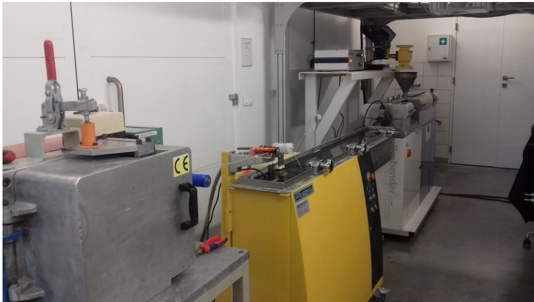
Figure 38: Lab-Compounder Brabender KETSE 20/40 with a cooling bath and a grinding mill
