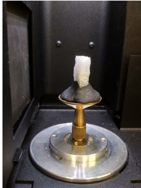
Figure 44: Attachment of the sample in Skyscan device
