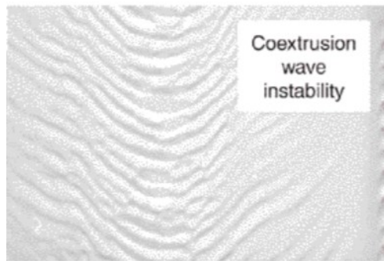
Figure 22: Interlayer instability wave pattern [32]
