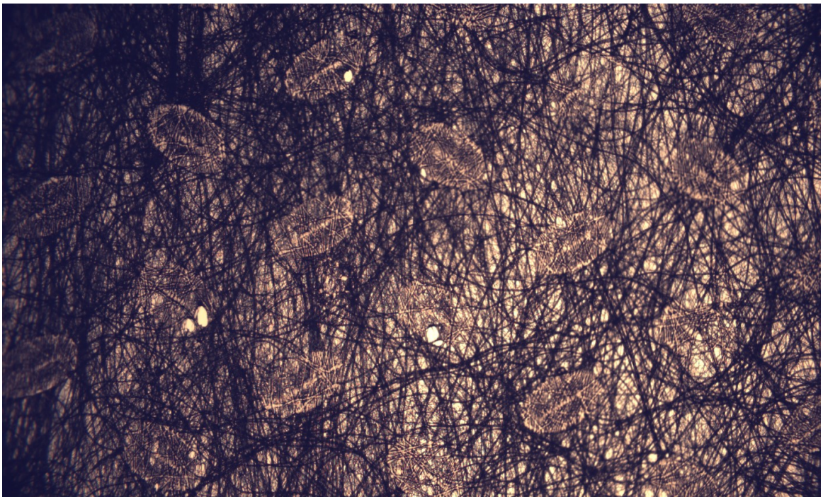
Figure 3 Spunbond nonwoven thermally bonded by calender
