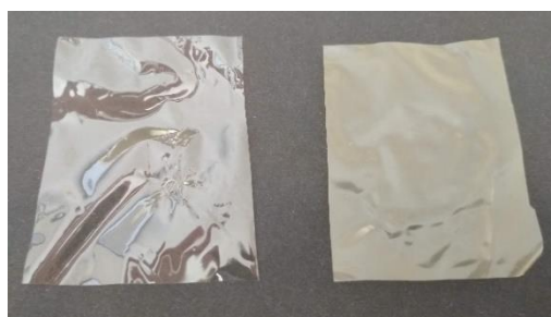
Fig. 12 Appearance of the chitosan films a) without and b) with thyme essential oil/Tween 80
