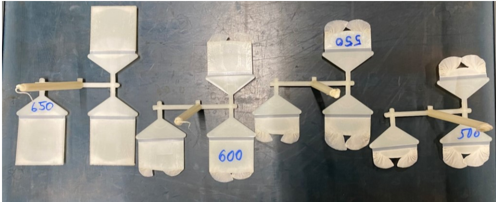
Figure 65 - Filling study of a three-cavity system (Ferromatik)
