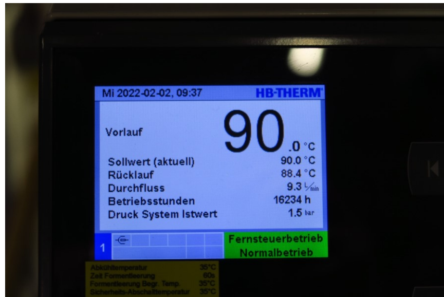
Figure 57 – Setting the tempering device (Demag)
