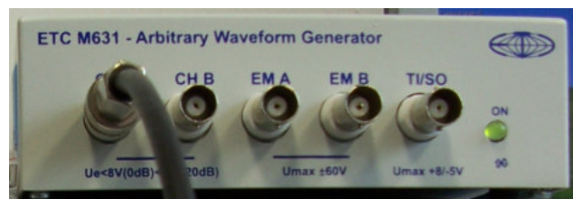
Figure 7: The basic parameters of the waveform generator.
