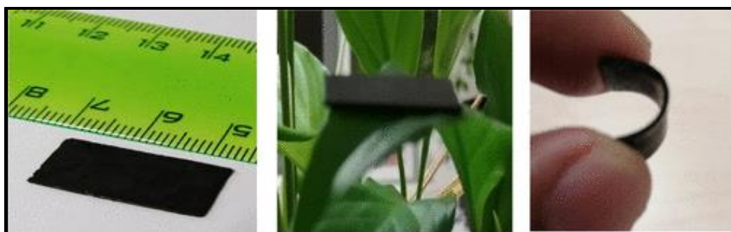
Figure 4.3 Pictorial representation of the developed TPU-based nanocomposite with spinel ferrite nanoparticles and reduced graphene oxide demonstrating the dimension, lightweight, and flexibility [A1].
