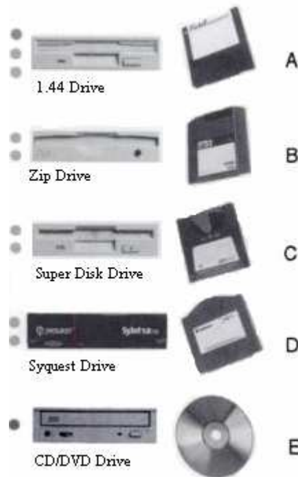
Fig. 2 The drives and input media
