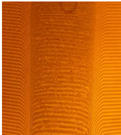
Figure 1 The example of interferogram illustrated diffusion proces sof swelling ( solid film of HA in KI solution at 35°C)
