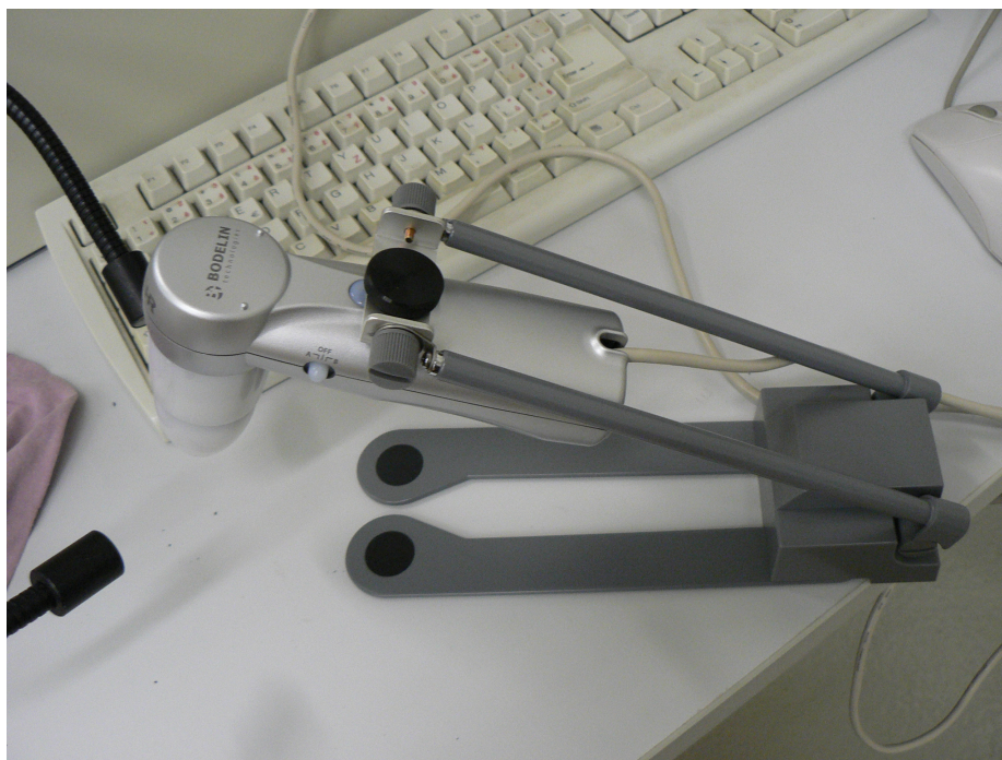
Obr. 17. PRESCOPE HR, Digital USB microscope
