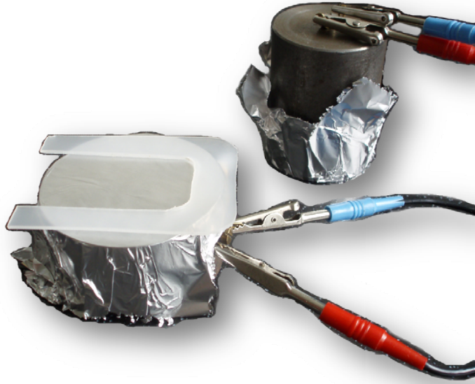
Fig. 20. Measuring electrodes covered by aluminum foil + plastic spacer
