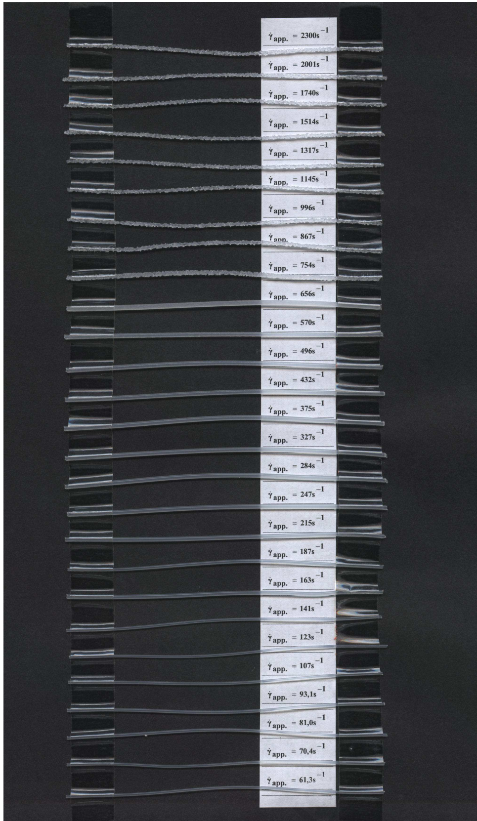
Fig. 49. Linear mLLDPE (low) extrudate samples obtained from orifice die ( L/D=0 , D=1 mm) at 140^{\circ}C for wide range of apparent shear rates ( 61.3-2300 s^{-1} )
