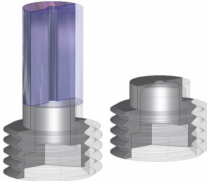
Fig. 19. Detail of long (left) and orifice (right) capillary dies
